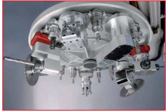
| 18-station tool changer of the BIMA 300
